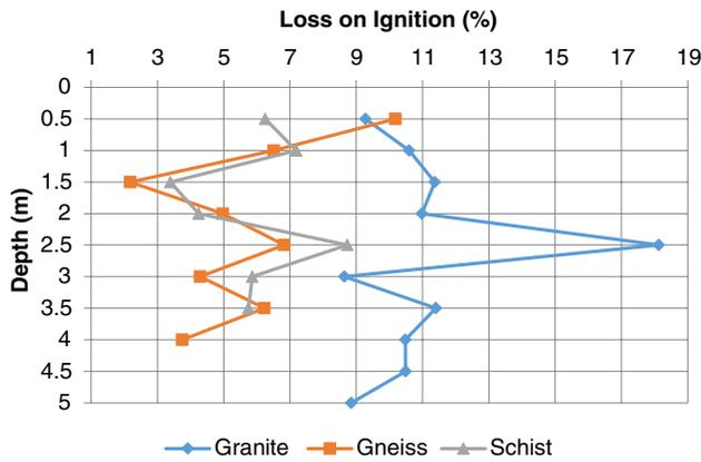
Fig. 8 Variation of loss on ignition with depth
