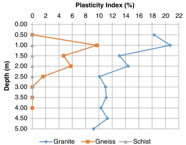
Fig. 10 Variation of plasticity index with depth
