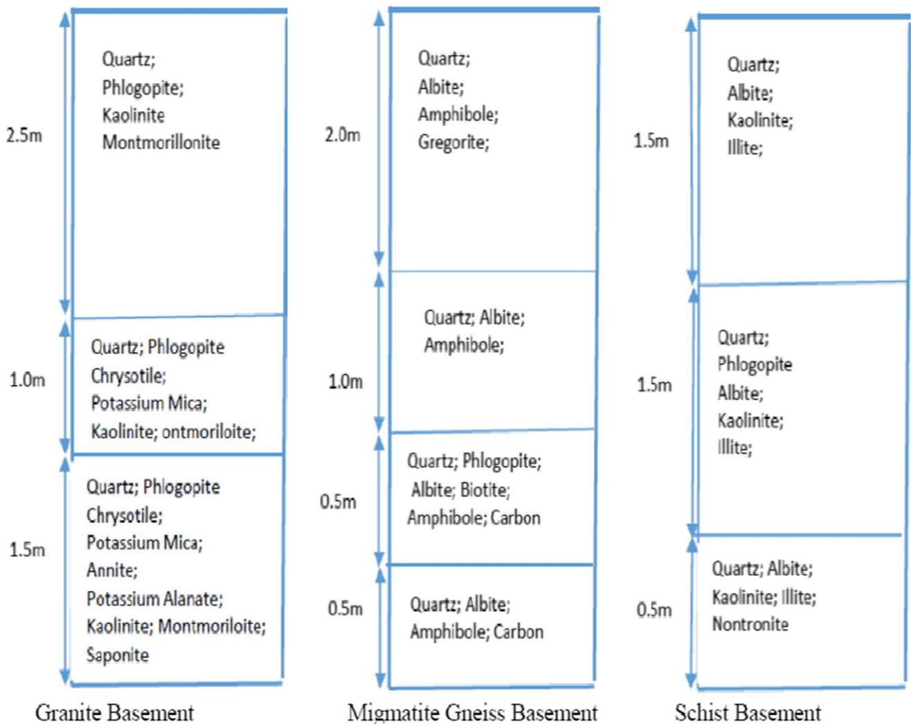
Fig. 13 Mineralogical groups forming layers in granite, migmatite gneiss, and schist basement complexes
