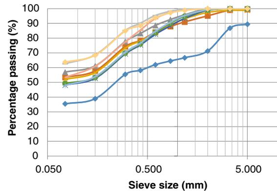
Fig. 11 Variation with depth of representative grain size distribution over granite
