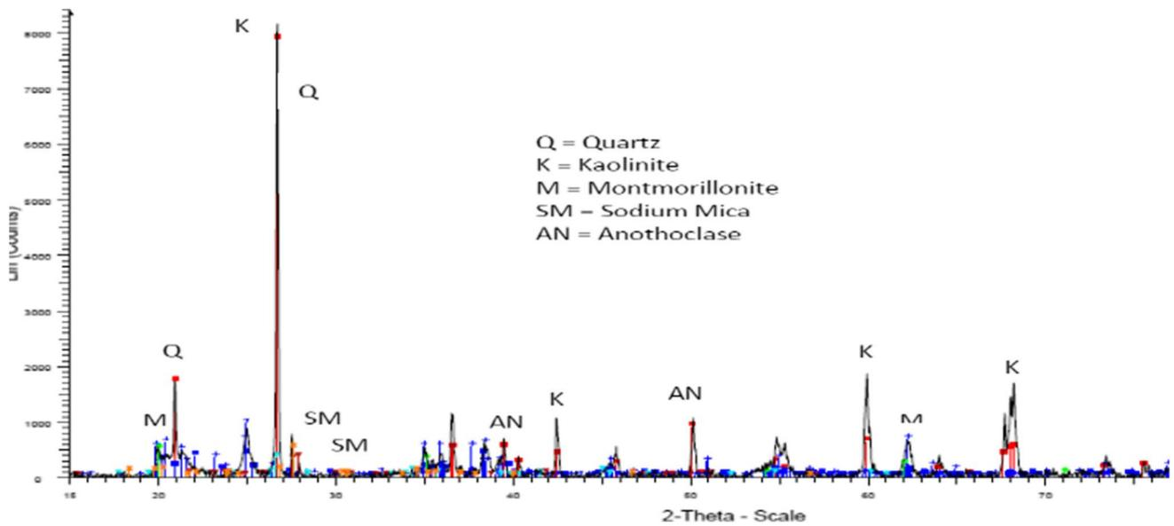
Fig. 2 Graph of representative XRD results for soils collected over granite basement at 0.5 m depth
