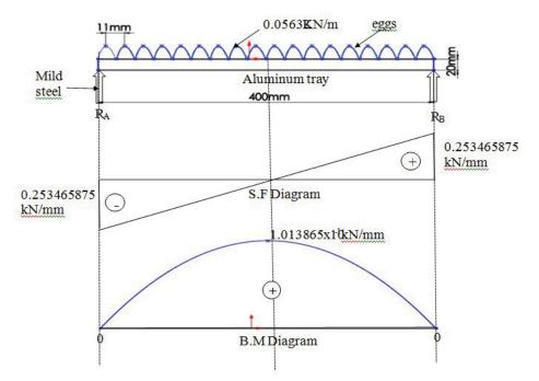
Figure 2: Bending Moment and Shear Force Diagram of the Load/Eggs on the Tray
