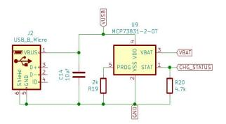
Figure 3: USB LiPo battery charging circuit
