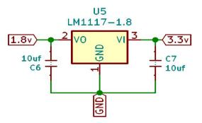
Figure 4: Voltage regulator circuit diagram
