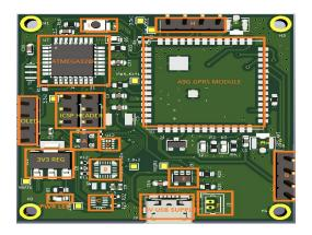
Figure 8: Front view of PCB
