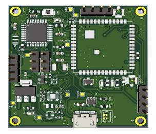
Figure 10: Test points for HR/BP Monitoring PCB
