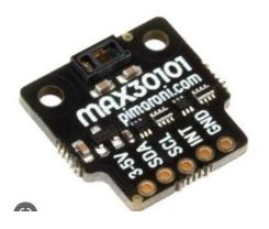
Figure 5: MAX30101 HR and BP sensor
