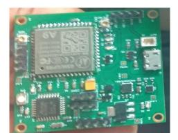
Figure 12a: HR/BP monitoring device (Front view)
