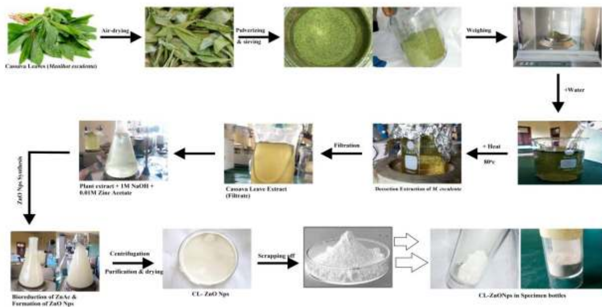
Figure 1: Process flow diagram for the synthesis of ZnO nanoparticle from cassava leaf
