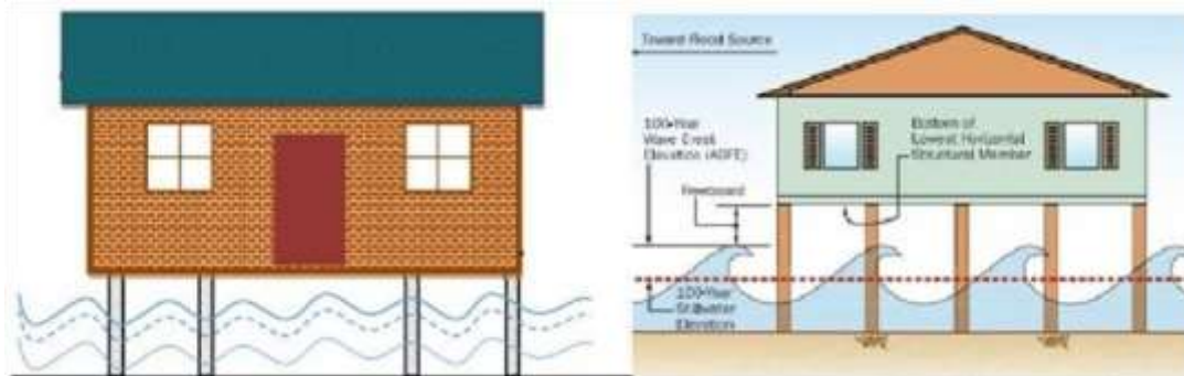
Figure III; Showing picture of elevated building structure along a flood plane and graphical illustration of the construction Source; Researchers' case study
