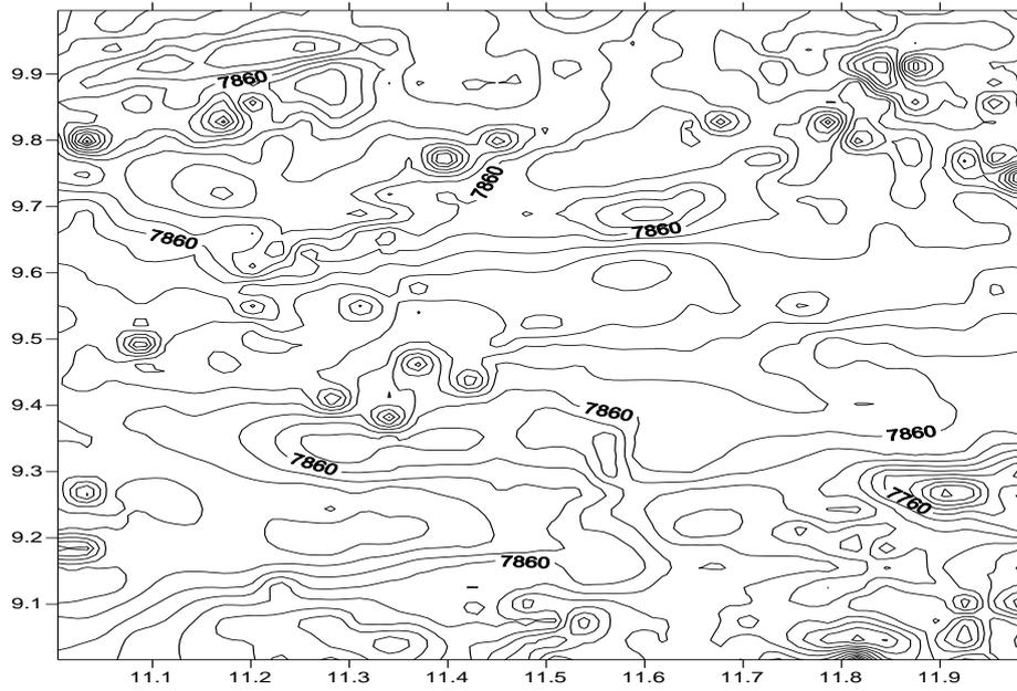
**Figure 4.1a: Total magnetic intensity contour map of the study area (Contour Interval = 20 nT)**
