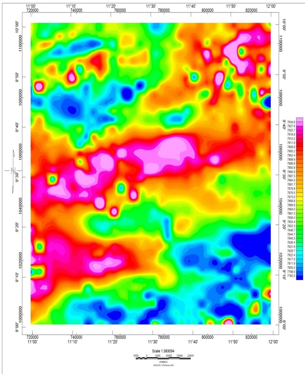
**Figure 4.4: Total magnetic intensity field of the area (normal flight height)**
