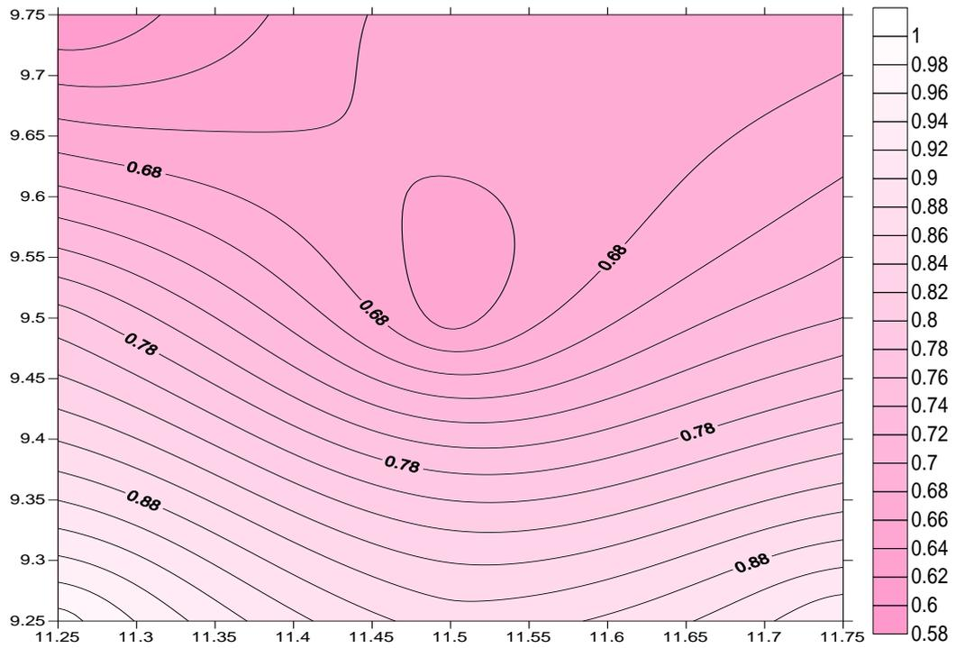
**Figure 4.14a: Contour map of first magnetic layer depth of the study area (Contour Interval = 0.02 km)**
