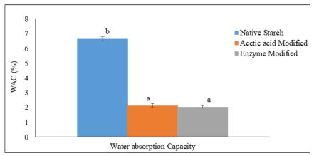
Figure 5: Water Adsorption Capacity of Native and Modified Cocoyam Starches
