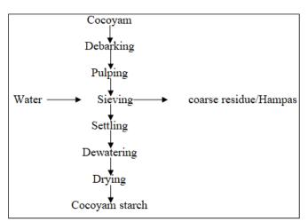
Figure 1: Schematic Flow Chart for Cocoyam Processing
