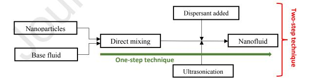
Fig. 2: One-step and two-step techniques of nanofluids preparation. Adapted and modified from Mirzaadi et al. (2021)
