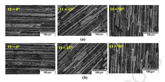
Fig. 3: SEM images of a machined surface obtained after milling operation (a) ACF vegetable oil conditions (b) dry (Adapted from Elgnemi et al., 2021)
