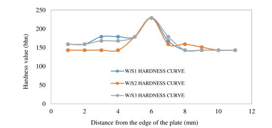
Figure 7: Variation of hardness value along the weld metal of sequence 1, 2 and 3
