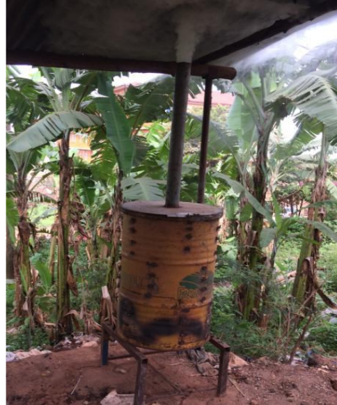
Figure 3.2: Carbonising kiln Source: (Kakooza, 2017)
