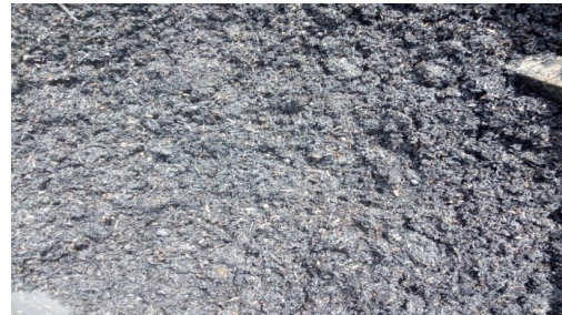
Plate IV: Carbonized rice husk mixed with binder
