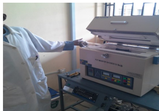
Plate 1: The horizontal CVD set up for the synthesis of carbon nanotubes
