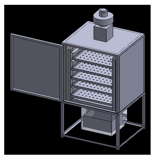
Figure 2.2: Cabinet dryer using sawdust briquette
