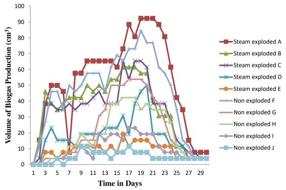
Figure 8: Variation of Volume of Biogas Production (cm<sup>3</sup>) with time
