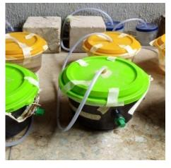
Figure 4: The Digester and the Gas Holder
