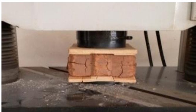
Figure 6: Compressive Strength test set up
