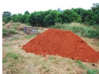
Figure 1: Laterite used for moulding interlocking blocks.
