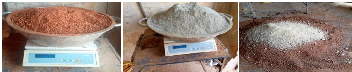
Figure 2: Batching of the materials.
