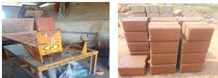
Figure 3. Hydraform interlocking blocks machine with single mould and blocks
