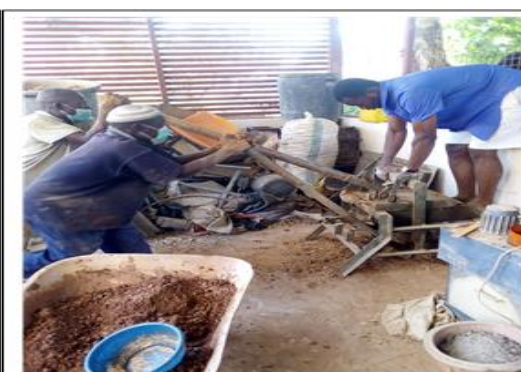
Figure 2 Compaction of contaminated stabilized soil mix
