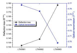
Fig. 3. Optical loss (R<sup>Loss</sup>) and optical transmission (T<sup>Opt</sup>) of the present investigated glassy samples).
