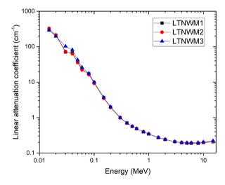
Fig. 4. Linear attenuation coefficient of the present investigated glassy samples.
