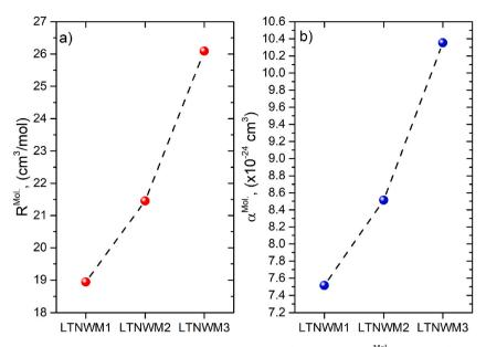
Fig. 2. Optical properties of the present investigated glassy samples (a) Molar refractivity ( $R^{Mol}$ ) and (b) Molar polarizability ( $\alpha_m$ ).
