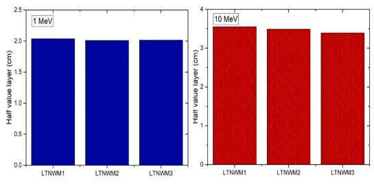
Fig. 7. Half value layer of the present investigated glassy samples at 1 MeV and 10 MeV.
