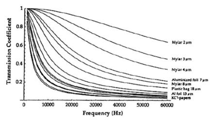
Figure 1 The acoustic transmission vs. foil thickness according to Vuohelainen (1998). Note the excellent resolution at 2–4 µm.
