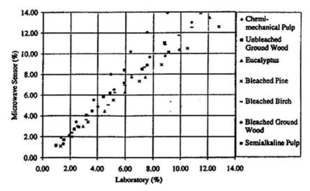
Figure 2 Consistency vs. microwave transmission.
