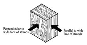
Figure 3 Design stresses for two product orientations.
