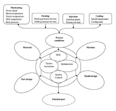
FIGURE 5.—Process parameters and critical factors influencing part quality in injection molding.
