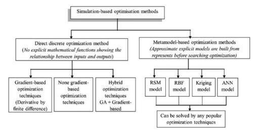
FIGURE 6.—Classification of simulation-based optimization techniques [1].
