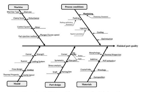
FIGURE 7.—The interactions of critical factors influencing part quality of injection molding products.
