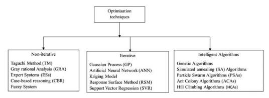
FIGURE 4.—Classification of optimization techniques used for injection molding process.
