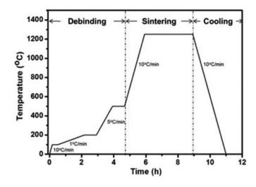
FIGURE 2.—Schematic of the thermal debinding and sintering processes [81].
