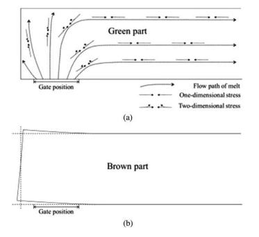
FIGURE 3.—(a) Possible flow path of melt in mold cavity generating internal stresses because of frozen-in orientation and (b) distortion of brown part due to stress relaxation [27].
