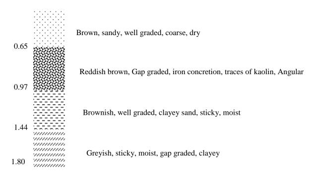
Figure 4.2 Typical Soil Profile at Lautech junction along the Road
