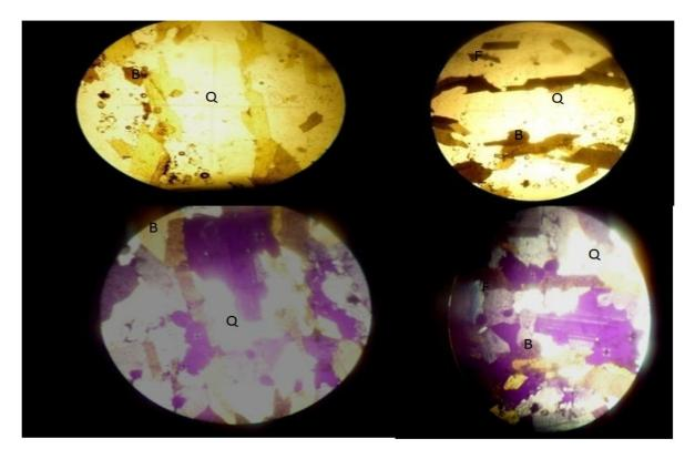
PLATE: III Mineral assemblage in thin section of the Migmatite (B= Biotite, Q= Quartz F= Feldspar; top two, under plane polarized light and last two cross polarized light)
