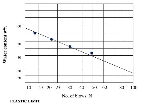
Flow index F1 = -28.7%Liquid limit = 50.0% Plastic limit =  $\underline{22.1\%}$ Plasticity index Ip=27.9% Toughness index = 1.0%
