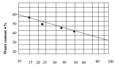
Flow index F1 = -26.2%Liquid limit = 52.5%Plastic limit = 26.5%Plasticity index Ip=26.0%Toughness index= 1.0%
