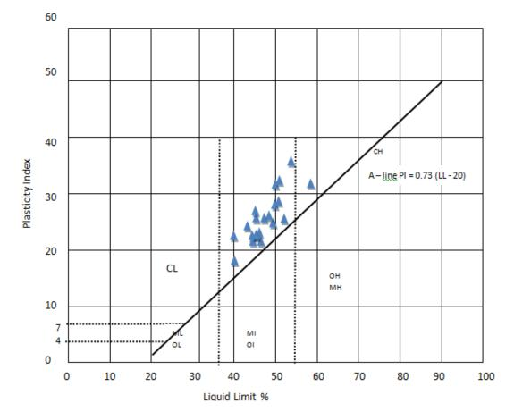
Figure: 4.3 Cassagrande soil Plasticity Chart for soil classification
