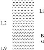
Light brown, clayey, fine, traces of kaolin, moist, poorly graded
