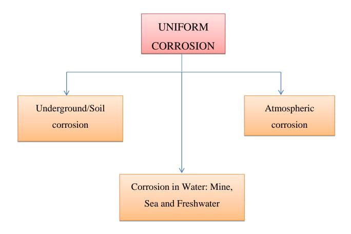
Figure 4. Types of uniform corrosion (Cicek, 2017).
