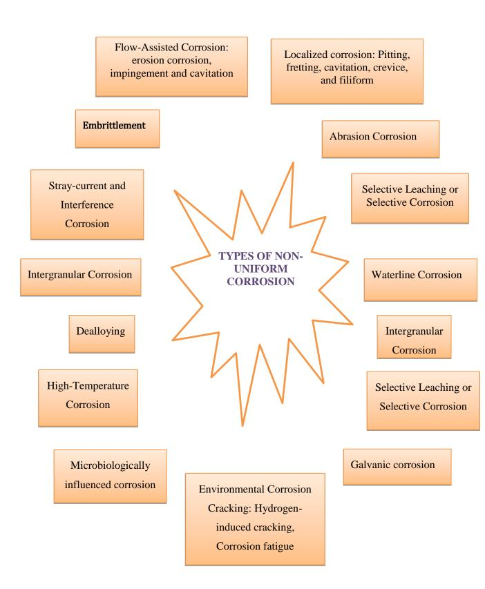
Figure 5. Various types of non-uniform corrosion compiled from Singh (2014) and Cicek (2017).
