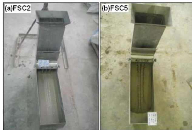
Fig 8. Examples of slump flow test: (a) FSC2, (b) FSC5.
