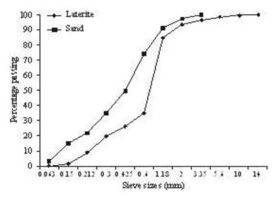
Figure 3: Grading curve for sand and laterite.
