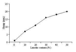
Figure 1: Slump of laterized concrete vs laterite .
