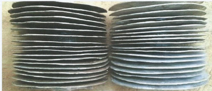
Figure 2. Aluminum heat sink fabricated for the present study
