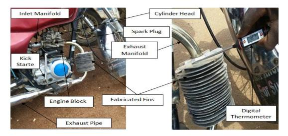
Fig. 1: Experimental Set-up and Testing
