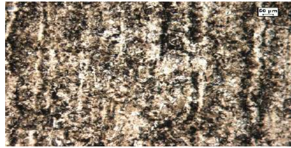
Fig. 6: Optical micrograph showing the microstructure of as-received 304 stainless steel.
