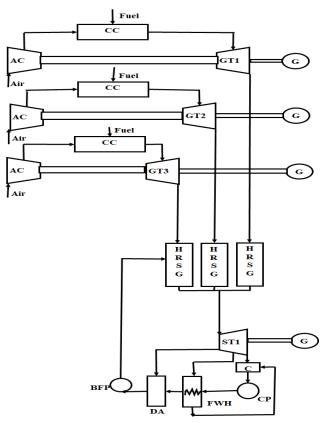
**Figure 2:** Model schematic diagram of the process flow of the CCPP at Afam VI power station
