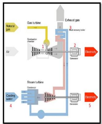
**Figure 1:** The basic principles of operation of a typical CCPP. (Source[<u>19</u>])
