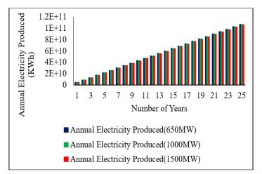
Figure 3: Annual electricity production for 650MW, 1000MW and 1500MW CCPP for 25 years period.
