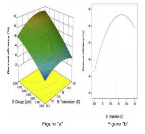
Figure 2: 3D Surface (a), and single effect (b) plot for effects of dosage ratio and reaction temperature on alumina removal from Obajana clay.
