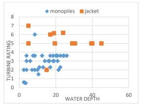
Figure 1. Graphical plot of turbine ratings (in MW) against water depths (in m) for OWTs supported on monopole and jacket foundations between years 2000 and 2018.
