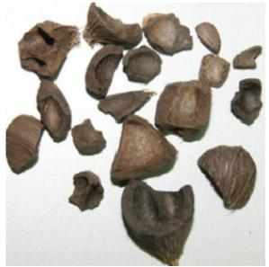
Figure 1: Palm kernel shell of various sizes
