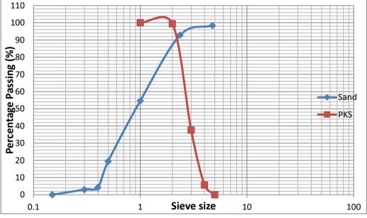
Figure 2: Sieve analysis of Sand and PKS
