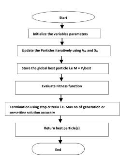
Figure 2. Particle Swarm Optimization model [34]
