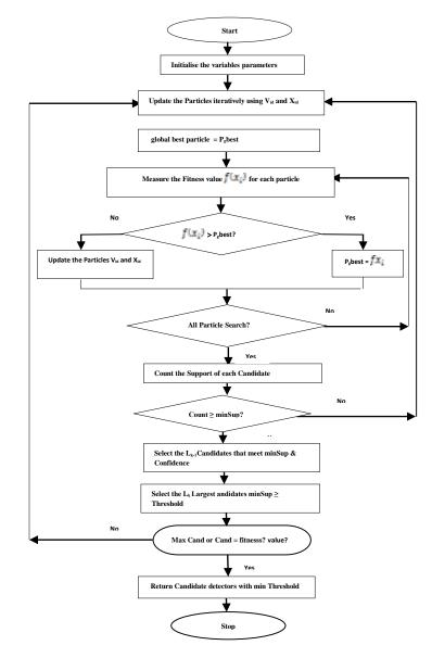
**Figure 3.** Proposed Improved AA-Particle Swarm Optimization candidate generation model
