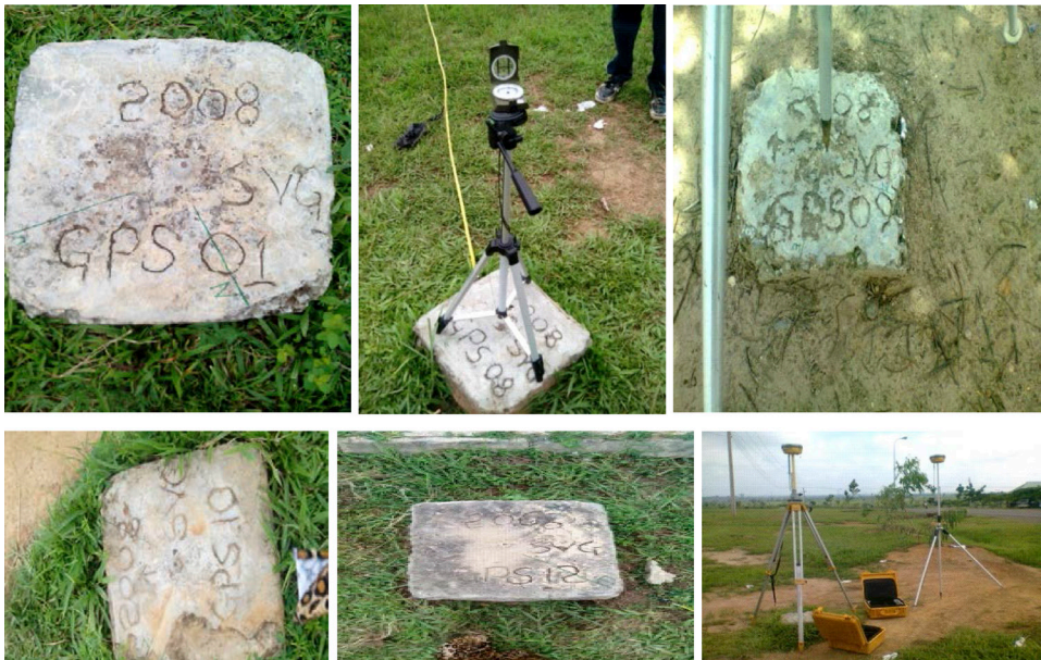
Fig. 3. Up – from left GPS 01, GPS 08 and GPS 09; down – from left GPS 10, GPS 12 and base station setup.
