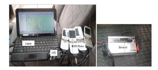
Figure 1. Drive test tools housed in a vehicle.
