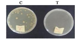
*P. aeruginosa* **Figure 7:** Evaluation of AgNPs as antimicrobial additives for detergent: C is the control (test organism and detergent only); T is the test (AgNPs-treated detergent and test organism).
