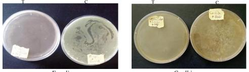
*E. coli C. albicans* **Figure 8:** Evaluation of AgNPs as antimicrobial additive for toothpaste: C is the control (test organism and toothpaste only); T is the test (AgNPs-treated toothpaste and test organism).
