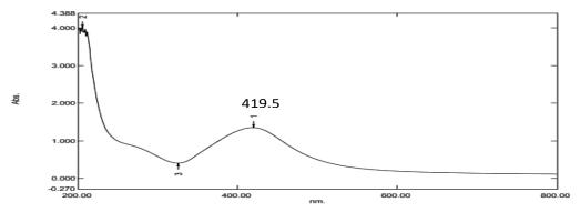
**Figure 3:** UV-Vis absorption spectrum of the biosynthesized AgNPs using aqueous stem bark extract of *A. occidentale*.
