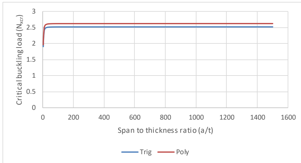
Figure 8: Graph of Critical buckling load ( N_{xcr} ) versus aspect ratio ( a/t ) of a rectangular plate with length to width ratio of 3.5
