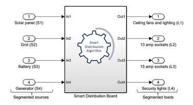
Figure 1. Smart distribution board model
