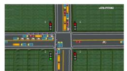
Fig. 11. Simulation showing green time signal for moving vehicles.
