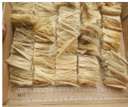
Figure 1: Treated Chopped Kenaf Fibre
