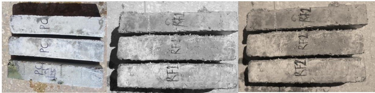
(a) 0% fibre concrete without RHA (b) 0.5% fibre and 5% RHA (c) 0.5% fibre and 15% RHA
