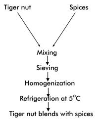
Fig. 2. Flow diagram showing the spiced tiger nut.
