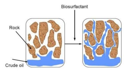
Figure 2.11: Mechanism of enhanced oil recovery by biosurfactants (Suthar et al., 2008)
