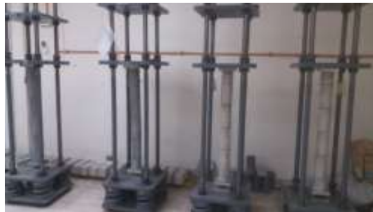
Figure 2: Compressive creep rig with specimen under sustained load
