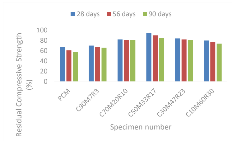
Figure 2: Strength losses as caused by H 2 SO 4 attack on ternary blended GPMs
