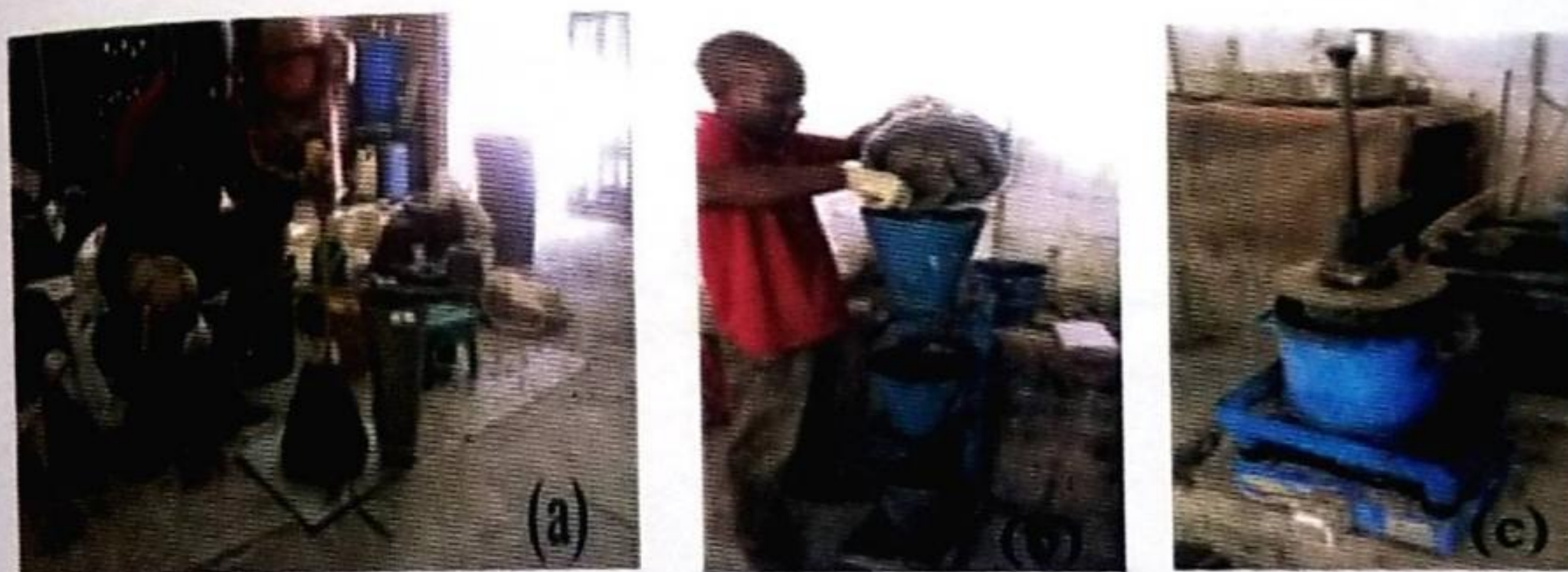
Figure 3: Measurement of (a) Slump, (b) Compacting Factor and (c) Vebe for workability test
