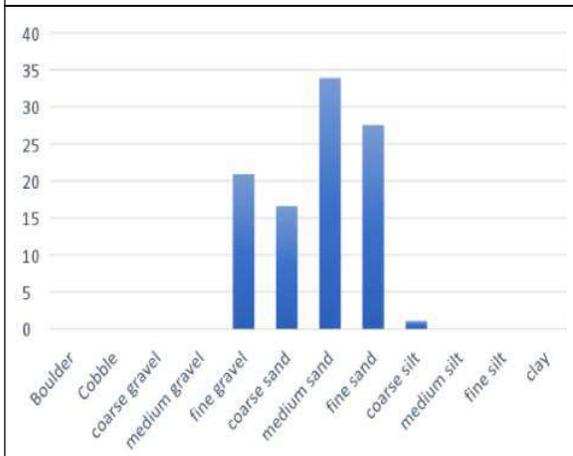
**Figure 14: Plot of Percentage Mass Passing (PMP) versus Siev Grain Size (Slump Site 5)**
