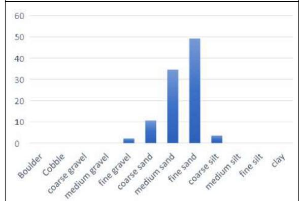
**Figure 16: Plot of Percentage Mass Passing (PMP) versus Siev Grain Size (Slump Site 6)**
