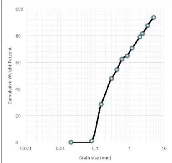
**Figure 11: Bar Chart Representation of Grain Sizes in Samples Slump Site 3**
