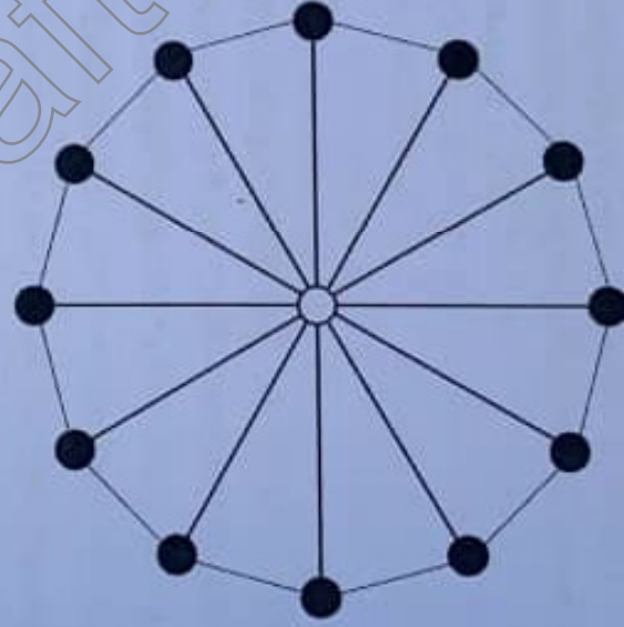
Figure 3: Layout of the Proposed Topology The topology is designed to offer path flexibility thereby eliminating single point of failure and reducing link congestion. With the availability of multiple path to the aggregator node for any SBS, Dijkstra algorithm is employed to route backhaul traffic using suitable Quality of Service (QoS) parameter as KPI. Since energy conservation is the outmost priority in this system, the system is designed to forward backhaul traffic
