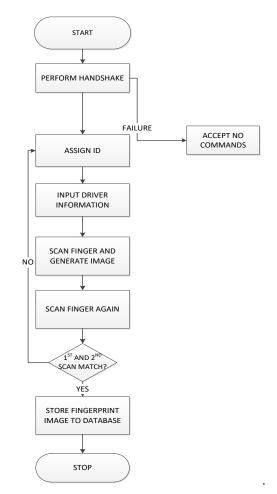
Figure 1. The Flowchart of the Enrollment Process
