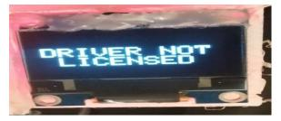
Figure 5. OLED Display of an Unregistered Driver
