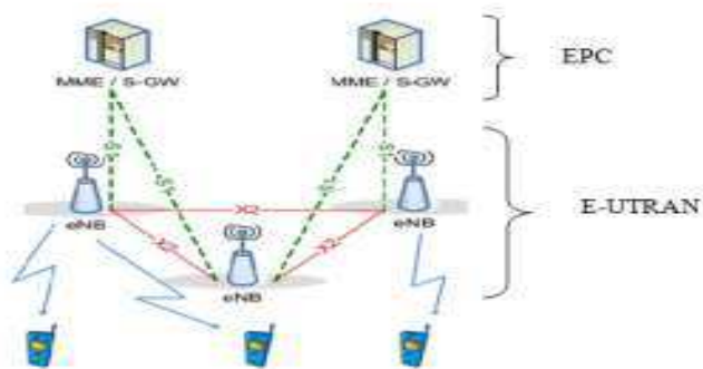
Figure 1: System Architecture of E-UTRAN
