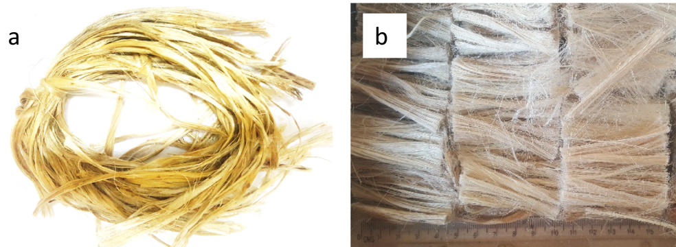
Fig 3 a Curl kenaf bio-fibre; b alkaline treated 50-mm length chopped kenaf bio-fibre
