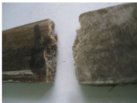
(a) Rupture section of KFRP composite sample.
