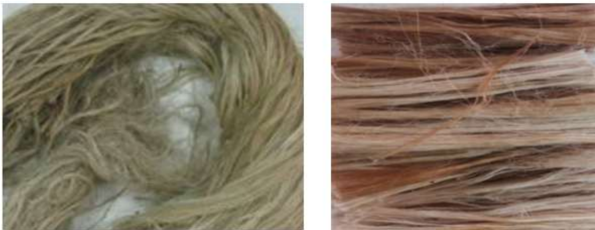
(a) Untreated Kenaf Fibre (b) 3 Hours Immersion of Kenaf fibre in 5% Alkali Solution
