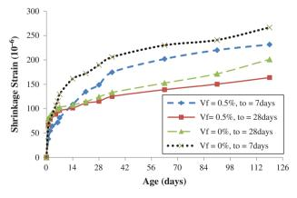
Fig. 5. Influence of fibre addition and age of exposure on the free drying Shrinkage of concrete,  $*t_o = exposure$  age of specimen to shrinkage testing.
