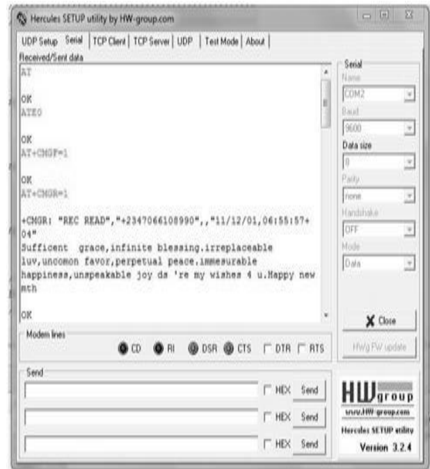
Figure 14: Screen shot of the Hercules setup utility of the Serial port to query the GSM modem
